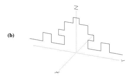
Fig.1 Geometry of the (a) Minkowski curve fractal of one iteration (M1) and (b) Minkowski curve fractal of two iterations (M2).
