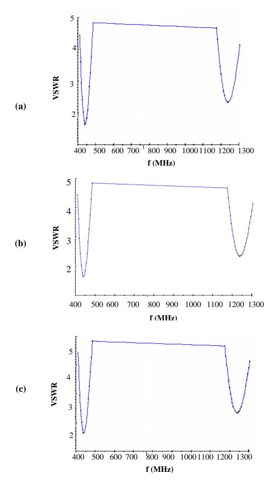
Fig.4 Voltage standing wave ration (VSWR)versus the frequency for the (a) HWD antenna, (b) M1 antenna, and (c) M2 antenna.
