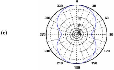
Fig.2 Radiation pattern at the resonant frequency of 440 MHz for the (a) half wavelength dipole (HWD) antenna, (b) M1 antenna, and (c) M2 antenna.
