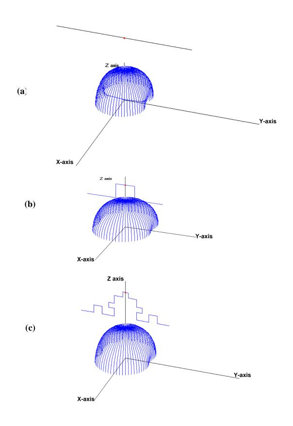
Fig.3 Three dimensions plot of the radiation pattern at the resonant frequency of 440 MHz for the (a) HWD antenna, (b) M1 antenna, and (c) M2 antenna.
